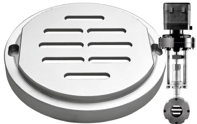
The slotted plates sliding against each other form the main throttling element in sliding gate valves. Since metal seats can be dispensed with in this system, scoring is eliminated which, in conventional valves, results very rapidly in expensive leaking.
