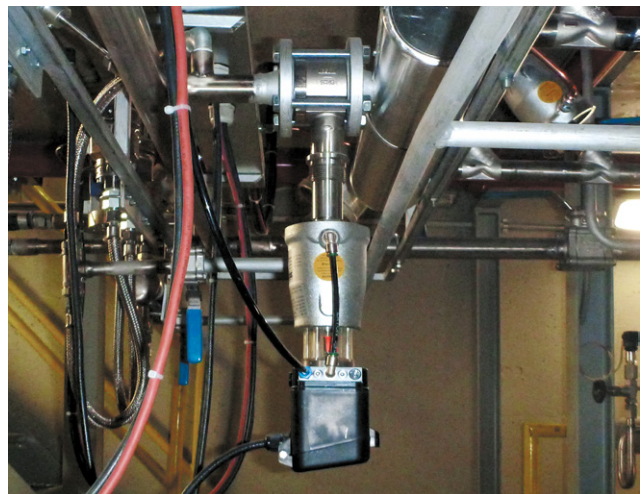
Angle seat valves and sliding gate valves on duty at Continental in Püchov.
