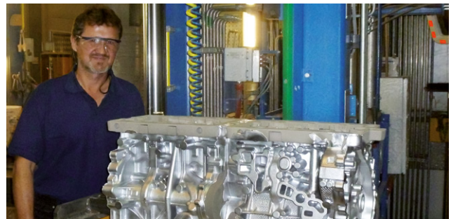
Casting: double-poured crank case
