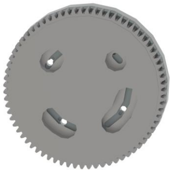
Fig. 2: Detailed view of the valve disc of the segmented disc valve in the desuperheater
